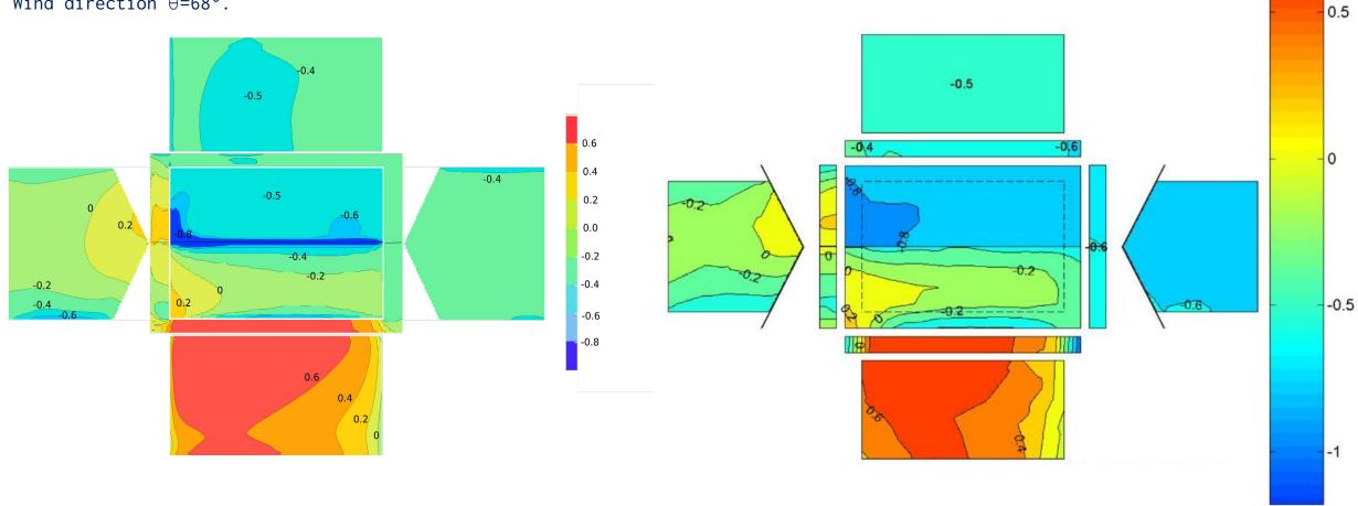
Pressure coefficient is calculated considering the wind pressure of the approaching wind velocity at the average roof height  $(0.5 \rho V_H^2, V_H^2)$  mean longitudinal wind speed at the reference height H,  $\rho$  the air density). The scales used for the comparison differ slightly in color shade.
